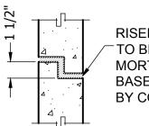
RISER SECTION TO BE SECURELY MORTARED TO BASE SECTION BY CONTRACTOR.
